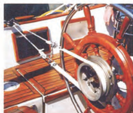
Wheel Adapter with Kevlar Belt
